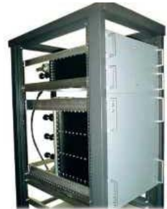
Example of rack-mounted combiners.
